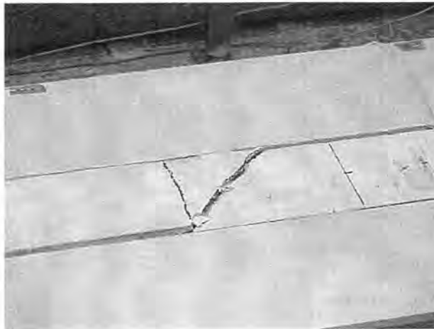
a. Photograph of partial composite behavior
