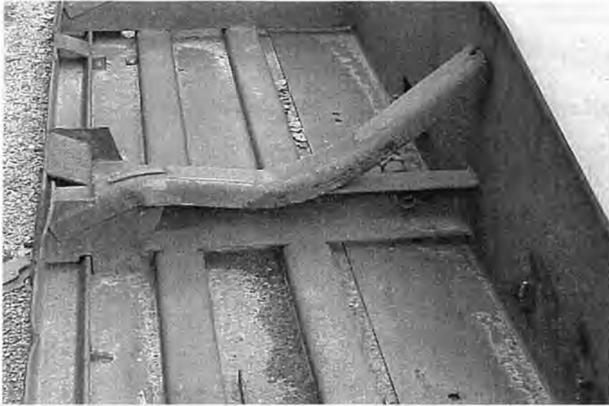
Figure 2.8. The deformed transverse member in AF4.
